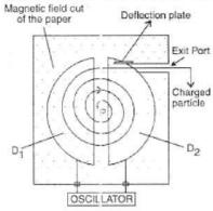
**Construction:** The cyclotron is made up of two hollow semi-circular discs like metal containers, D<sub>1</sub> and D<sub>2</sub> called dees.
